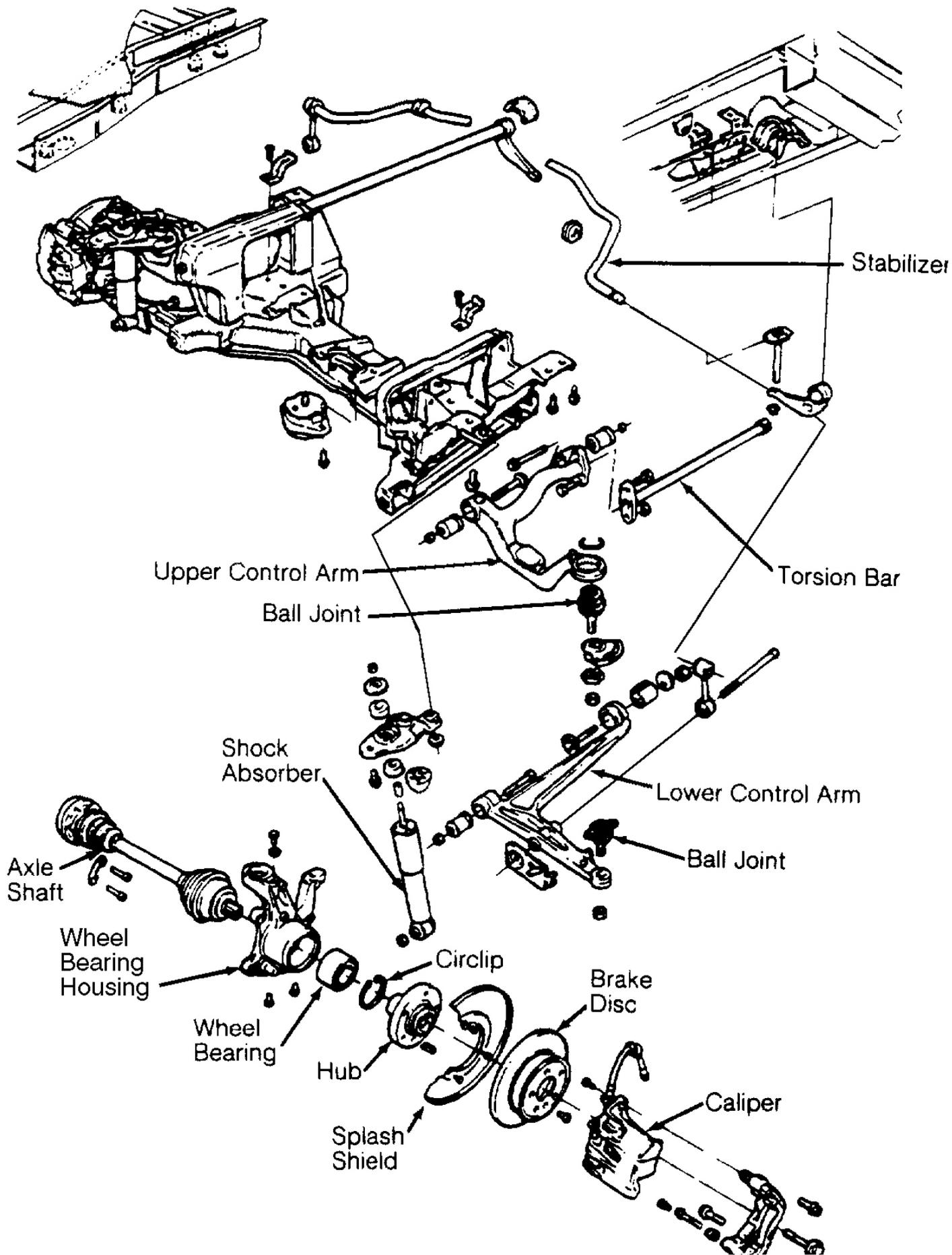
**Fig. 1: Exploded View Of Front Suspension**
